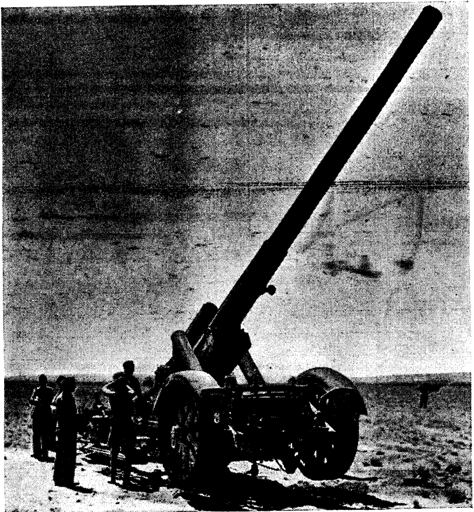
Figure 41.—170-mm gun (17 cm Kanone in Mörser-Lafette 18).
